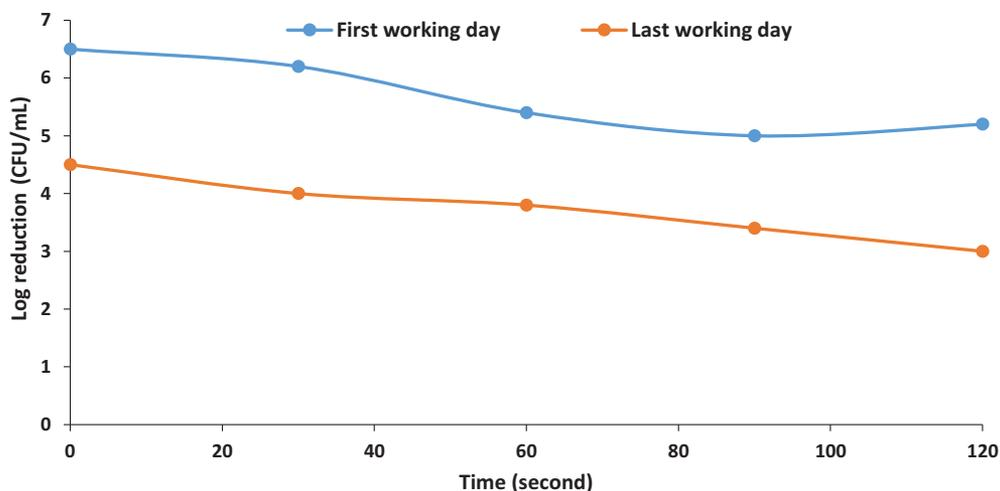
**Figure 1.** The effect of flushing (without ozone) on reducing the microbial load at different times.
