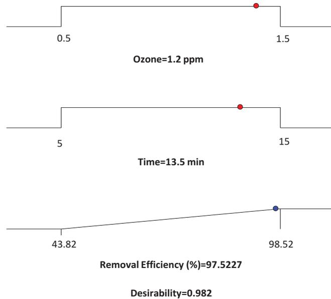
**Figure 5.** Desirability ramp for optimization of DUWLs disinfection process.
