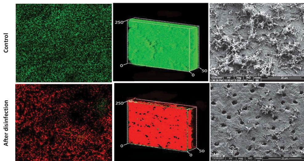
**Figure 6.** CLSM and SEM images of bacterial biofilm before and after disinfection by ozone.
