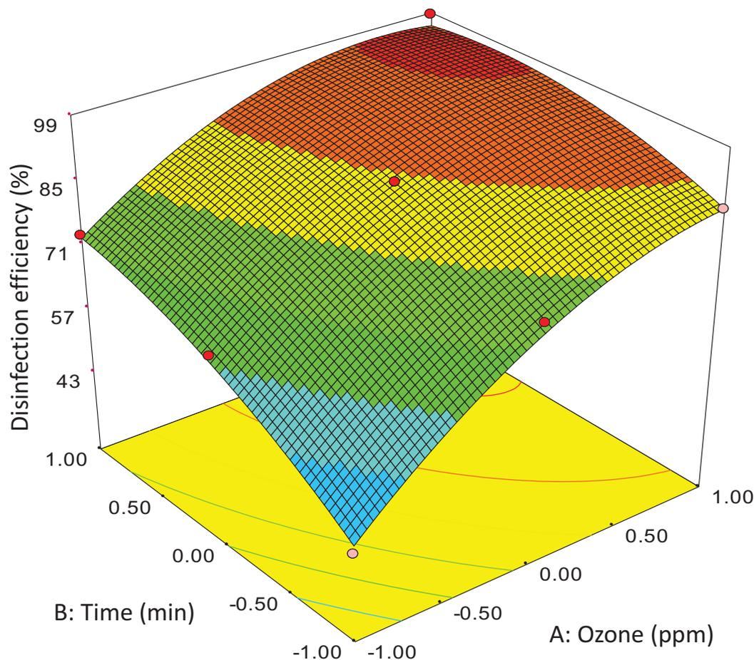
**Figure 4.** Contour plot showing the interactive effect of the initial concentration of ozone and reaction time on DUWLs disinfection.
